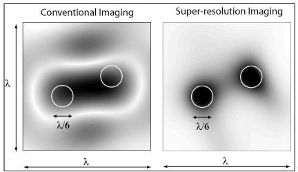
Experimental demonstration of subwavelength resolution imaging with ultrasound. The resolution of conventional imaging methods is affected by the Rayleigh diffraction limit, super-resolution techniques overcome the limit and resolve two subwavelength cylinders (diameter  $\lambda$  /6) revealing details smaller than the wavelength,  $\lambda$ . Simonetti et al. PRE 76 2007.
