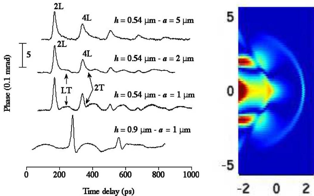
“Measurement of elastic stiffnesses of (sub-) $\mu\text{m}$  films by picosecond ultrasonics”
