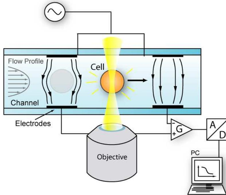
“Microfluidic chips for high speed multiparameter particle analysis: applications in genomics”
