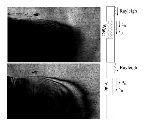
Figure 6.20: The upper 82MHz SAW amplitude image is of a 1° sub-surface slit, with the void behind the slit filled with water. At least one of the Lamb modes is severely dampened in this case by the water. The lower image is of the same region on the sample, but with the water drained out.
