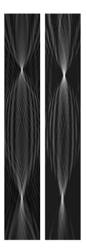
Figure 3.11: Predicted (a) and measured (b) SAW amplitude distributions at 82MHz produced by the hybrid continuous wavefront/DAE shown in figure 3.10. Image size is  $0.8 \times 6.4$ mm.
