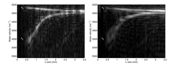
Figure 6.12: Fast Fourier transform (FFT) of the complex amplitude of the SAWs propagating over the 1° slit. The left hand image is from the data acquired by propagating a plane wave, the right hand image is from the data acquired by propagating a focused wave, and is identical to figure 6.6. The  $a_0$  and  $s_0$  modes are labelled.
