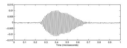
Figure 4.14: A typical simulated detector signal used to test the AAPD.
