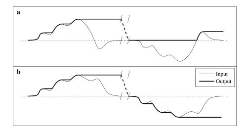
Figure 4.8: Expected outputs from (a) a unipolar peak detector, and (b) a bipolar peak detector.
