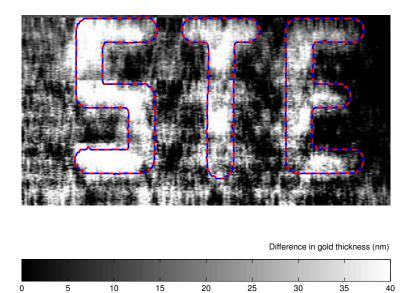
Figure 5.16: Image representing the difference in gold thickness at different points on the area shown. An outline of the mask edges has been artificially added for clarity. The size of the image is  $14 \times 7.2 \text{mm}$
