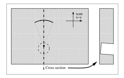
Figure 6.18: Schematic of the 'hole experiment.' A 1mm diameter hole is drilled into base of a piece of polished aluminium at an approximate 1° angle. The sample is scanned in the x-y directions to achieve a normal c-scan. The vertical dimension and slit angle in the cross-section diagram have been greatly exaggerated.
