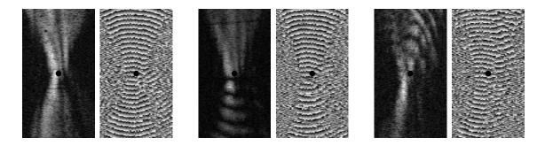
Figure 6.9: Amplitude and phase aerial PSFs at three scan positions for the c-scan shown in figure 6.5. The left hand PSFs are for a position above (i.e. before) the slit. The centre pair of images are for a point just on the boundary of the upper edge of the slit and the thick aluminium. The right hand PSFs are for a point on the slit itself. The small circle in the centre of each image indicates the location of the detection point.
