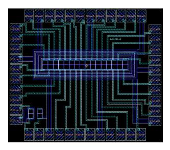
Figure 7.16: Design for a 16-channel optical acoustic wave front sensor (AWFS).
