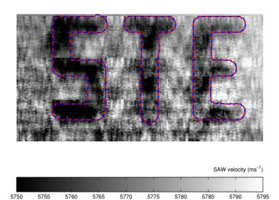
Figure 5.15: SAW velocity image, acquired from the filtered phase information shown in figure 5.14. The size of the image is  $14 \times 7.2$ mm
