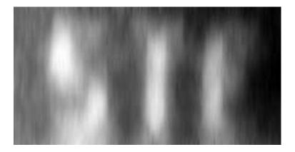
Figure 5.14: 82MHz SAW phase image, covering the same area as figure 5.13b, spatially filtered in the direction of propagation (vertical). The size of the image is  $14 \times 7.2$ mm
