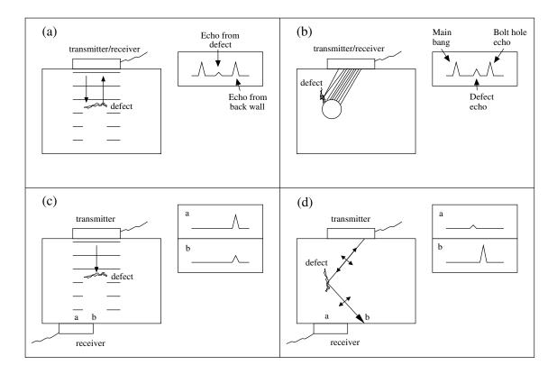
Figure 1.1: Illustrations of the four main techniques of detecting flaws in the interior or materials: (a) reflection, normal beam; (b) reflection, angle beam; (c) transmission, normal-beam; (d) transmission, angle beam. The type of signals received relating to the defect are shown as inserts.
