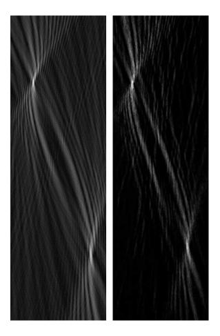
Figure 3.18: Predicted (a) and measured (b) SAW amplitude distributions at 82MHz produced by the hybrid continuous wavefront/DAE shown in figure 3.17. Image size is  $2 \times 6.4$ mm.
