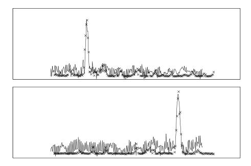
Figure 3.19: Predicted (-) and measured (×) amplitude through the two 82MHz foci.
