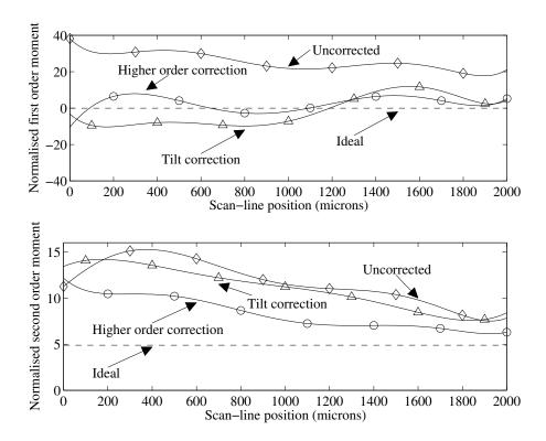
Figure 7.14: The upper plot shows normalised first order moments of the acoustic intensity for uncorrected  $(\diamond)$ , tilt-corrected  $(\triangle)$  and higher-order-corrected  $(\diamond)$  line-scans. The ideal (--) is also shown. The lower plot shows the second order moments of the same data. Both plots are best-fit lines through experimental data.
