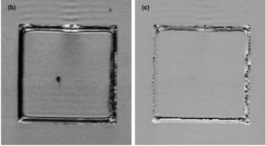
Figure 8.6: Optical (a), 82MHz SAW amplitude (b) and phase (c) images of an aluminium-coated sample. The area inside the square is designed to be poorly bonded to the substrate.
