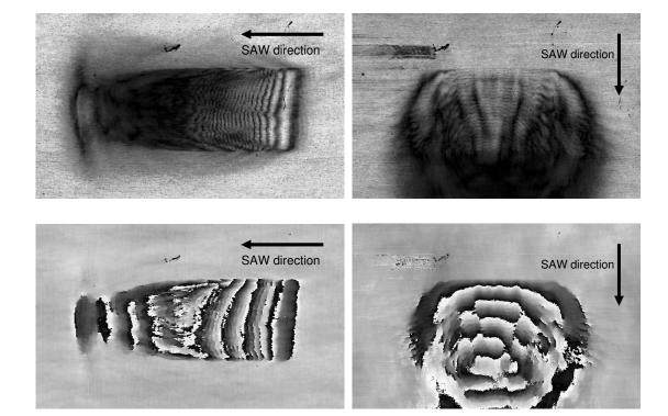
Figure 6.17: SAW 82MHz amplitude (top) and phase (bottom) images of the 'circular profile slit' shown in figure 6.15. In the left hand images, the SAWs are travelling from right to left, as indicated by the arrow. In the right hand images, the SAWs are travelling from top to bottom. The left hand images are  $7.5 \times 4.5$ mm, the right hand images are  $7 \times 4.5$ mm.
