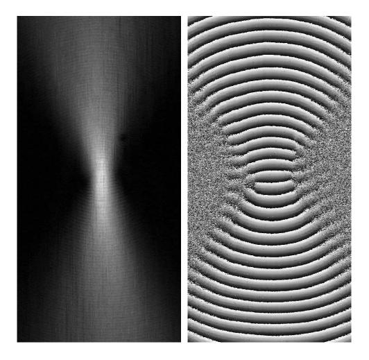
Figure 3.3: Amplitude (left) and phase (right) aerial point spread functions produced from a source of concentric arcs. The images were obtained using the O-SAM on an 'ideal' sample, by scanning the detection point relative to the generation arcs and the sample. The image size is  $0.5 \times 1$ mm, and each pixel represents an area of  $2 \times 1 \mu$ m.
