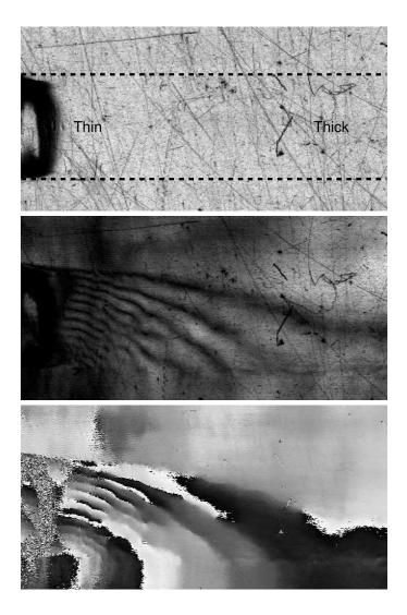
Figure 6.5: Optical (top), 82MHz SAW amplitude (centre) and 82MHz SAW phase (bottom) c-scan images of a  $3.5 \times 1.75$ mm area of the top surface of a piece of polished aluminium. The location of the slit is shown by dashed lines in the optical image. The slit breaks the surface on the left of the image, where the thickness of the aluminium is at its thinest.
