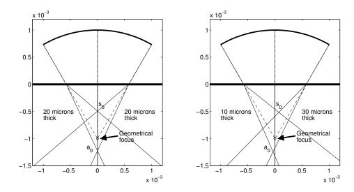
Figure 6.8: The left hand image illustrates the effect of attempting to focus SAWs though a boundary between uniform thick and thin layers. The faster  $s_0$  waves come to a focus before the geometrical focus, whereas the  $a_0$  waves come to a focus after it. The right hand image illustrates the additional effects of propagating through a medium of varying thickness along the x-direction; the foci are now displaced in the x-direction also.
