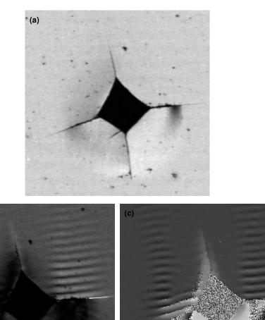
Figure 8.5: Optical (a), 82MHz SAW amplitude (b) and phase (c) images of the Vickers hardness indentation on silicon nitride, previously presented in figure 5.4 in chapter 5. Some of the features of the acoustic images are difficult to interpret.
