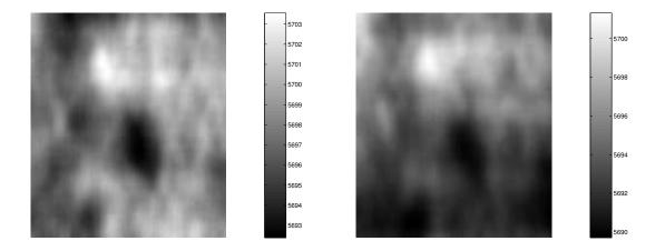
Figure 5.7:  $11.5 \times 16$ mm mean velocity images of a silicon nitride sample. The left hand image is derived from 82MHz SAW phase, the right hand image is derived from 164MHz SAW phase. The source  $\rightarrow$  detector separation is 2mm, and the data has been spatially filtered to approximately this resolution.
