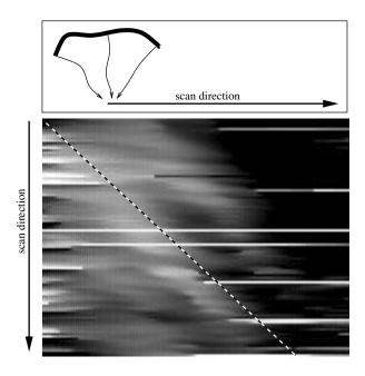
Figure 7.15: The upper schematic diagram indicates the wavefront propagation and scanning directions. The intensity of the lower image represents the phase errors (horizontal axis) for each point along the scan-line (vertical axis). The added diagonal dashed line indicates the position of a reference point. Size of image is 2.6mm×2mm.
