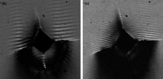
Figure 5.4:  $0.8\times0.8$ mm images of a Vickers hardness test indentation on a silicon nitride sample. The three images are as follows: (a) optical image; (b) 82MHz SAW amplitude image; (c) 164MHz SAW amplitude image. The resolution is  $1\times1\mu$ m
