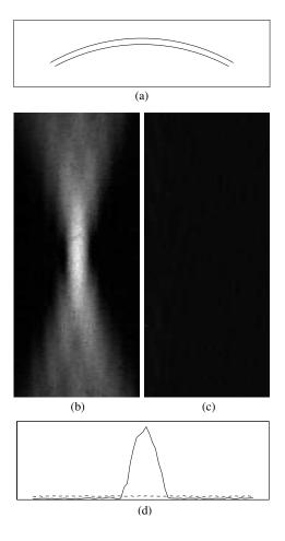
Figure 3.6: Realisation of a surface acoustic wave band stop filter (a), that retains the fundamental frequency of 82MHz inherent in the optical excitation energy and removes the 164MHz harmonic. (b) and (c) show the aerial PSFs at 82MHz and 164MHz respectively. (d) is a line plot through the focus at both frequencies. Aerial PSF size is  $600 \times 300 \mu m$ .
