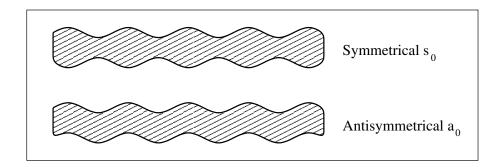
Figure 6.1: Representation of the first symmetrical  $(s_0)$  and antisymmetrical  $(a_0)$  Lamb wave modes. The amplitude of the waves is significantly exaggerated in the figure for illustration purposes.
