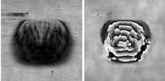
Figure 6.15: Optical (top), 82MHz SAW amplitude (lower left) and 82MHz SAW phase (lower right) images of a  $7 \times 7$ mm area of the top surface of a piece of polished aluminium. The location of the slit is shown by dashed lines in the optical image. The slit is thinest at the centre (horizontally) of the image.
