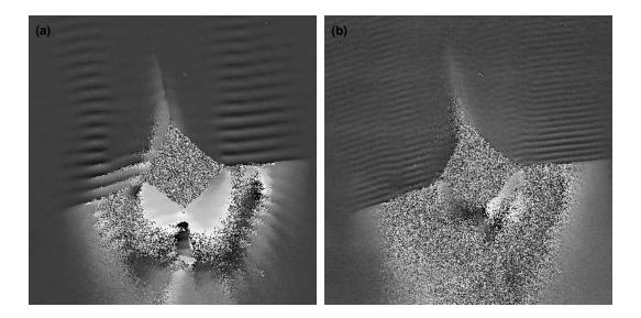
Figure 5.5:  $0.8 \times 0.8$ mm SAW phase images of a Vickers hardness test indentation on a silicon nitride sample, covering the same area as the images in figure 5.4. (a) 82MHz SAW phase image; (b) 164MHz SAW phase image. The resolution is  $1 \times 1 \mu$ m
