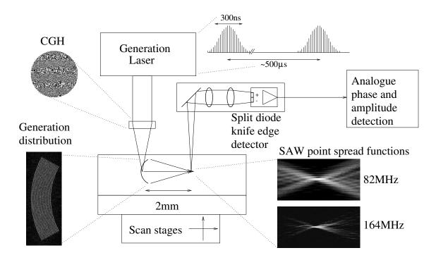
Figure 3.1: Block diagram of the all-optical scanning acoustic microscope (O-SAM).
