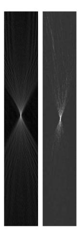
Figure 3.12: Predicted (a) and measured (b) SAW amplitude distributions at 164MHz produced by the hybrid continuous wavefront/DAE shown in figure 3.10. Image size is 0.8×6.4mm.
