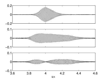
Figure 3.8: The first trace was obtained from the focus of an arc acoustic element and shows no envelope broadening. The second trace was obtained from the focus of the diffractive element shown in figure 3.7. The third trace was obtained from just above the focus of the diffractive element, within a 'dark lobe.' The horizontal scale denotes time in  $\mu$ s since Rayleigh wave excitation.
