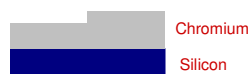
Figure 7 Schematic of sample showing stepped chromium layer, thin region c . 50nm, thick region c . 70nm.
