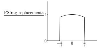
Figure 4.6: Plot of the transverse light distribution  $\Pi_{ab}(\mathbf{r})w(\mathbf{r})$ , where w has a <u>PSfrag replacements</u> Gaussian envelope.
