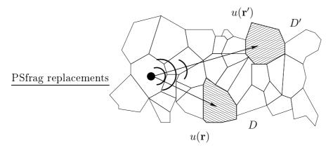
Figure 2.1: The correlation of the field at two different grains in polycrystalline materials.
