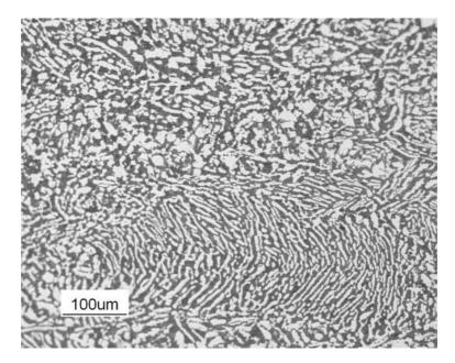
Figure 6.5: Photomicrograph of the surface of titanium etched by standards procedures to reveal the microstructure.
