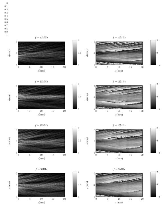
Figure 6.13: Amplitude and phase distribution of the acoustic field  $u(\mathbf{r}, \omega | \gamma)$  showing aberrations in titanium at different frequencies. The propagation is from left to right. The right side column shows the amplitude of the field whereas the other column the residual phase.
