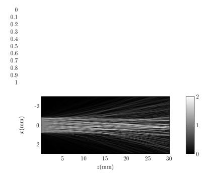
Figure 4.7: Amplitude distribution according to Eq. (4.17). The simulation is based on real parameters and a numerical procedure. This can be compared with the experimental amplitude distribution shown in Fig. (1.1).
