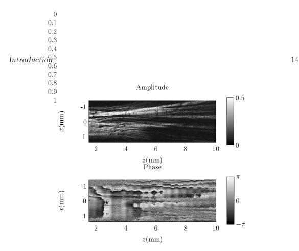
Figure 1.1: The image on top is the amplitude distribution A whereas the image on bottom is the phase distribution  $\Phi$  of a plane wave at 82MHz, travelling from left to right on an aluminium sample. The two images were obtained with OSAM system.
