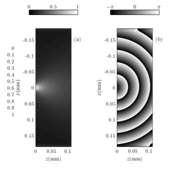
Figure 4.2: a) Amplitude of the complex normal displacement (arbitrary units). b) Phase distribution (radians)
