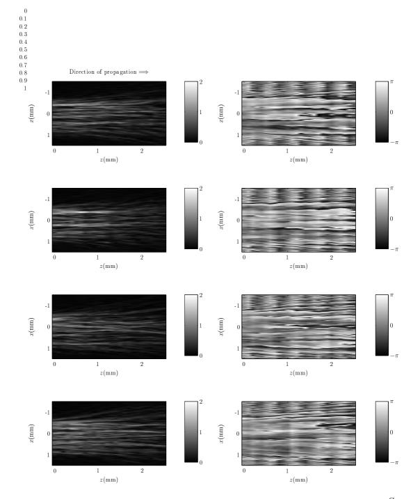
Figure 6.12: The right column is an image of the amplitude distribution of  $u_n^C$  at different instances across the sample C. The second column shows an image of the phase distribution for each field to left. The wave propagates from left to right as indicated by the arrow on top of the first column.
