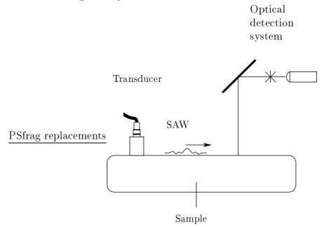
Figure 2.2: Simplified representation of a typical experimental setup SAW generation using a transducer as source of ultrasound. The detection system can vary but it could be used the knife-edge detection system.
