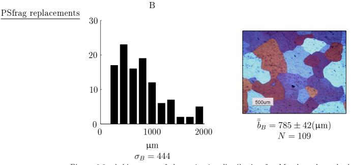
Figure 6.3: A histogram of the grain size distribution for  $M_B$  showed on the left hand side, where  $\sigma_B$  is the standard deviation of the grain size distribution. To right hand side, the photomicrograph of aluminium sample is shown, under-cross polarised.
