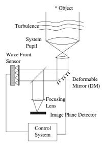
Figure 1.3: A simplified optical configuration of an adaptive optical imaging system, redrawn from [1].
