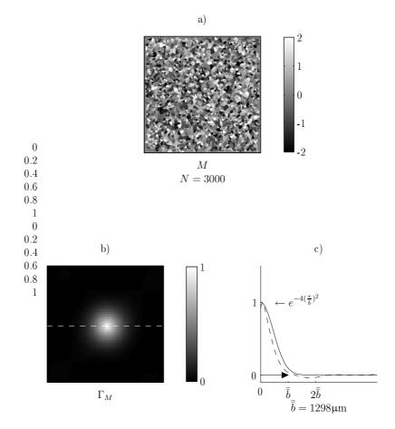
Figure 3.6: a) Simulated microstructure using Voronoi cells. b) The two-dimensional Fourier transform of M normalised to maximum value. c) Comparison of the transverse correlation function  $\Gamma_M$  as indicated by the dashed line in (b) to  $\Gamma_{\mu} = e^{-4\frac{\tau^2}{l^2}}$  to obtain l or  $\overline{b}$ .
