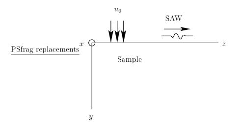
Figure 3.2: Geometry of SAW in polycrystals. The vertical arrows pointing downwards indicate the location of the initial field displacement  $u_0$ . The horizontal arrow is indicating the direction in which a SAW propagates.
