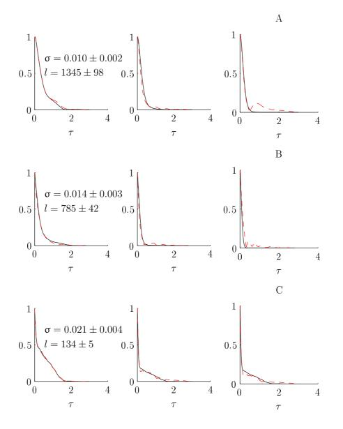
Figure 6.16: Comparison of theoretical and experimental correlation functions,  $\Gamma_u$  and  $\Gamma_e$  for the three blocks A, B, C of aluminium. The dashed lines is  $\Gamma_e$  at several distances whereas the continuous line is  $\Gamma_u$  at same distances. The half-width of the plotted functions is proportional to mean grain size. The numerical values for  $\sigma$  and l are given for each of the three cases.
