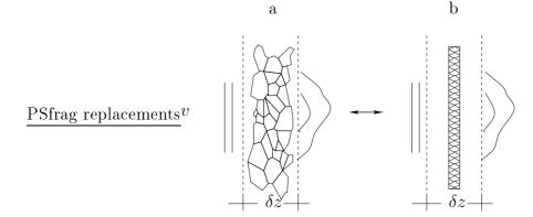
Figure 4.3: Schematic representation of ultrasonic propagation in a random medium using phase screen theory.
