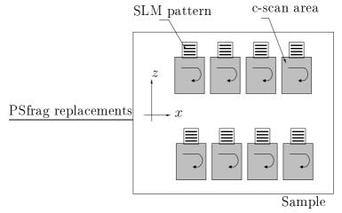
Figure 6.8: Schematic representation of scanning area and source locations to built up an ultrasonic ensemble. At each position of the SLM, marked with a series of black and white stripes, a c-scan was performed across x and z direction. The direction of propagation is along the z axis.
