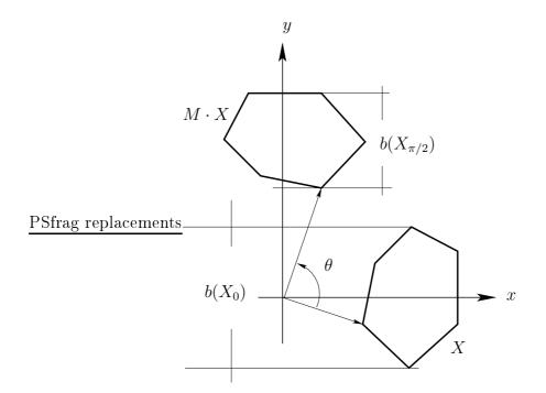
Figure 3.3: Rotation of object X around zero, which represents grain around. The matrix M rotates X by an angle  $\theta$ , the calliper diameter is the distance between the points intersecting the vertical axis as indicated by  $b(X_0)$  and  $b(X_{\pi/2})$ .
