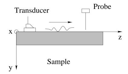
Figure 6.7: Sample and transducer array for SAW generation. The probe and the whole detection system in this experimental setup correspond to the OSAM system.
