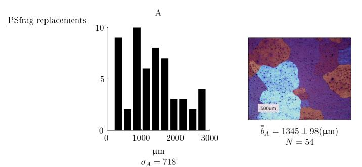
Figure 6.2: A histogram of the grain size distribution for  $M_A$  is showed on the left hand side, where  $\sigma_A$  is the standard deviation of the grain size distribution. To the right hand side, the photomicrograph of the aluminium sample is shown, under-cross polarised.
