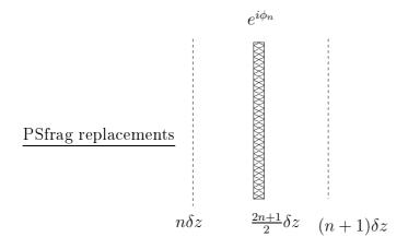
Figure 4.4: Schematic representation of the *n*th layer replaced by the phase screen system. The screen  $s = e^{i\phi_n}$  is being allocated in the middle of the layer.
