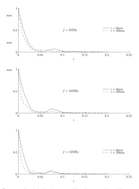
Figure 6.17: Correlation function measured from the acoustical ensemble in titanium showing the decay at different frequencies and distances. The dashed lines correspond to  $\Gamma_e$  whereas the continuous ones correspond to  $\Gamma_u$  at different distances.
