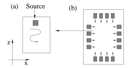
Figure 6.9: (a) Area in xz plane which c-scan has been performed. (b) The black square represents the multiple positions where the transducer has been located to perform a c-scan according diagram (b); whereas arrows indicate the direction of propagation.
