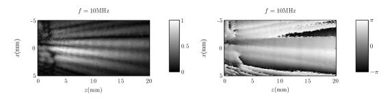
Figure 6.14: Amplitude and phase distribution of the acoustic field at 10MHz on an ideal sample (Glass) with no microstructure. The transducer output is not a single beam as one might expect.
