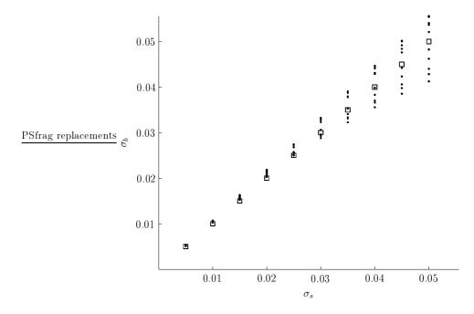
Figure 6.19: Comparison of the best value  $\sigma_b$  (dots on the graph) on simulated microstructure. The symbol  $\sigma_s$  stands for the standard deviation used to simulate the medium. The plot is a comparison between the standard deviation estimated by solving the minimisation problem Eq. (6.4), for the simulated acoustic fields in a simulated media with standard deviation  $\sigma_s$ , represented by a small square.
