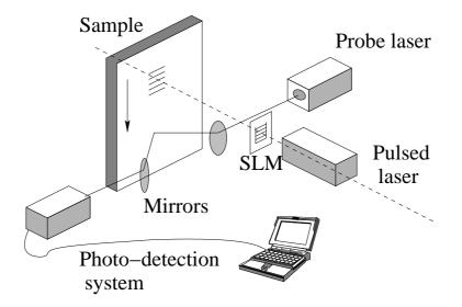
Figure 6.6: A pattern generated by a spatial light modulator is imaged onto the sample using a pulsed laser. This pattern acts as the source of the surface acoustic waves. The waves are detected by another laser, using an optical beam deflection technique [19].
