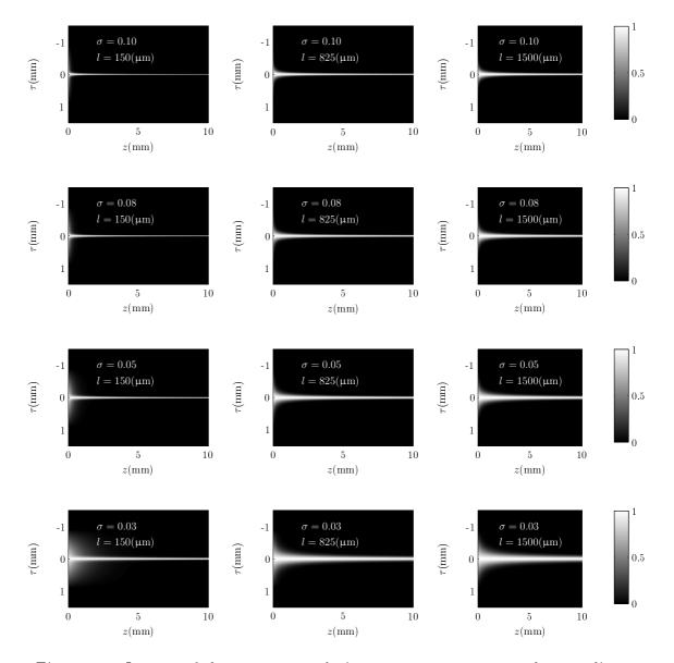
Figure 5.3: Images of the energy correlation propagating in a random medium -z-direction- as a function of  $\sigma$  and l, Eq. (5.21). The correlation function has been plotted in arbitrary normalised units.
