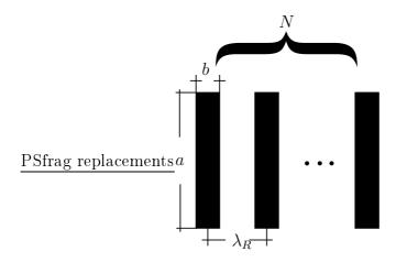
Figure A.1: Array of N illuminated lines by a laser. a, b are the width and length, respectively of the lines and  $\lambda_R$  is the Rayleigh wavelength which is the distance of separation between adjacent lines.
