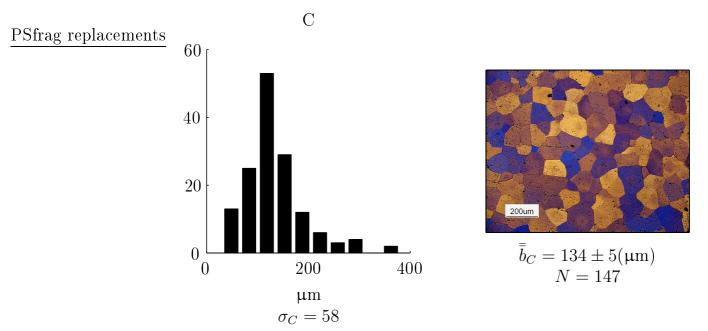
Figure 6.4: A histogram of the grain size distribution for  $M_C$  showed to the left hand side, where  $\sigma_C$  is the standard deviation of the grain size distribution. To right hand side, is the photomicrograph of the aluminium sample showing, under-cross polarised light the grain for block  $M_B$ .
