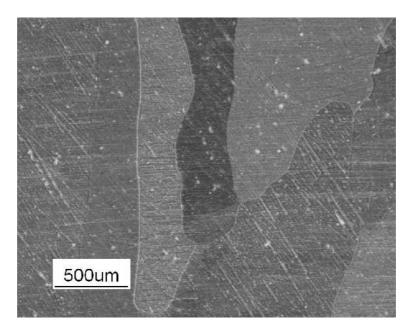
Figure 6.1: Photomicrograph showing individual elongated grains in an aluminium sample. The photomicrograph was obtained in a conventional microscope under cross-polarised light.
