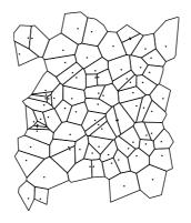
Figure 3.4: The Poisson Voronoi tessellation simulating microstructure of polycrystals. Only a few regions are being showed for illustration purposes. The dots inside the regions are the seeds from which regions are grown.
