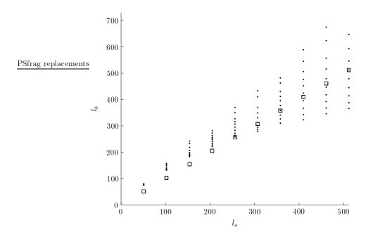
Figure 6.20: Comparison of the best value  $l_b$  (dots on the graph) on simulated microstructure. The symbol  $l_s$  stands for the mean grain size used to simulate the medium. The plot is a comparison between the correlation length  $l_b$  estimated by solving the minimisation problem Eq. (6.4), for the simulated acoustic fields in a simulated media with average grain size  $l_s$ , represented by small squares.
