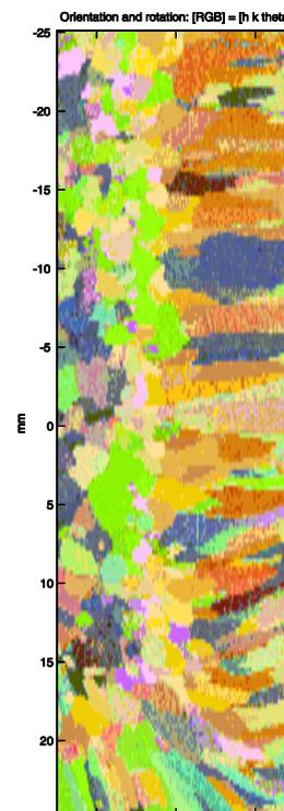
**Figure 7- Orientation map of large grain aluminium sample**
