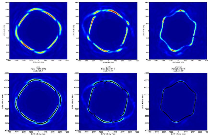
**Figure 6 Top - experimental data on 3 single crystal nickel samples. Lower - data overlaid with the best fit modelled data.**
