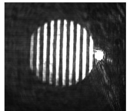
Figure 4 image of the grating pattern on the sample surface
