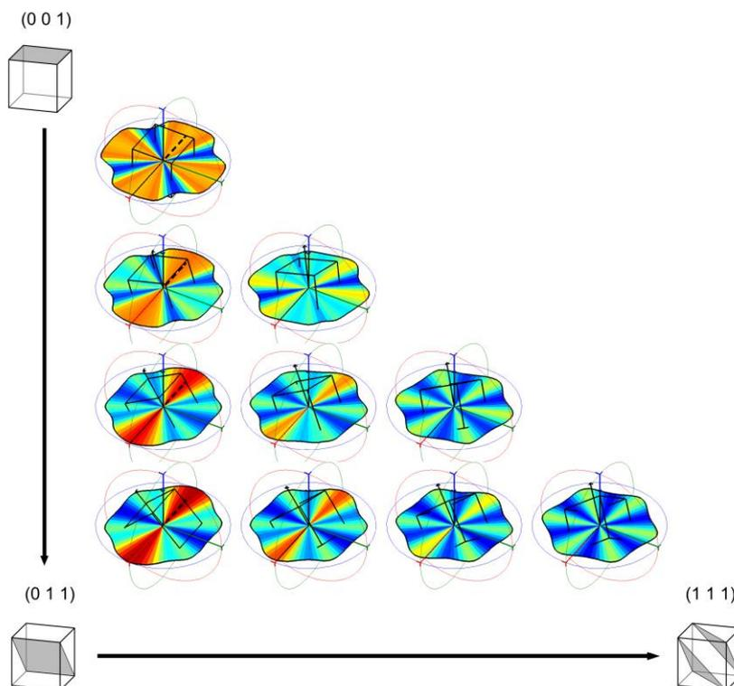
Figure 5 - Calculated velocity surfaces for Nickel
