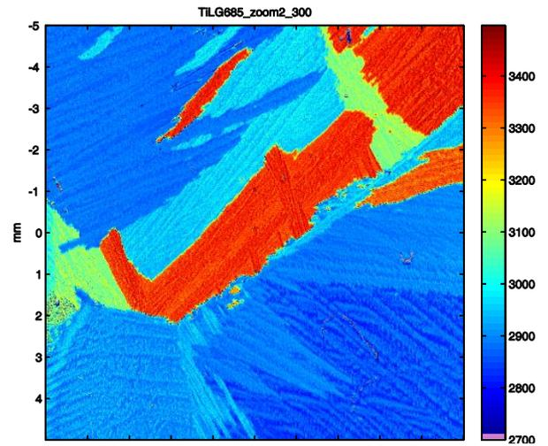
Figure 3 - High resolution SRAS scan
