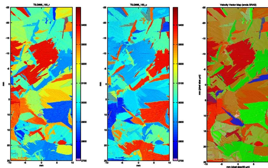
Figure 4 Saws propagating left/ right (left) up /down (centre) and a velocity vector map combining both (right)
